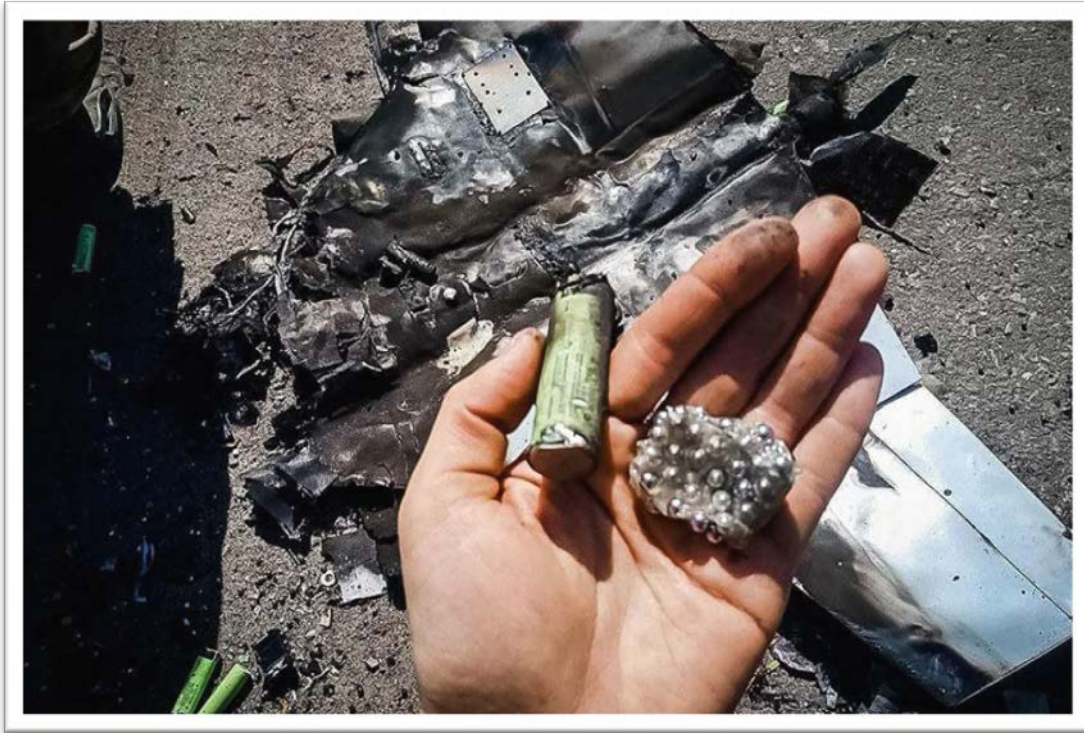
Figure 31 – A Ukraine soldier shows the steel balls used in the KYB’s antipersonnel round
