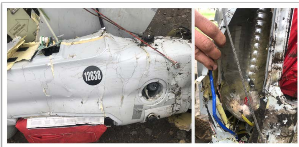
Figure 18 - An Orlan-10 crashed on 24 April 2022. Its fuel tank appears to be a recycled water bottle
