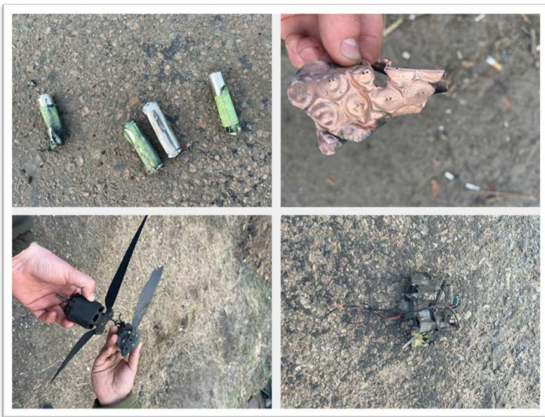
Figure 30 – Debris from a Zala Aero KYB UAV that detonated over a command post in Luhansk
