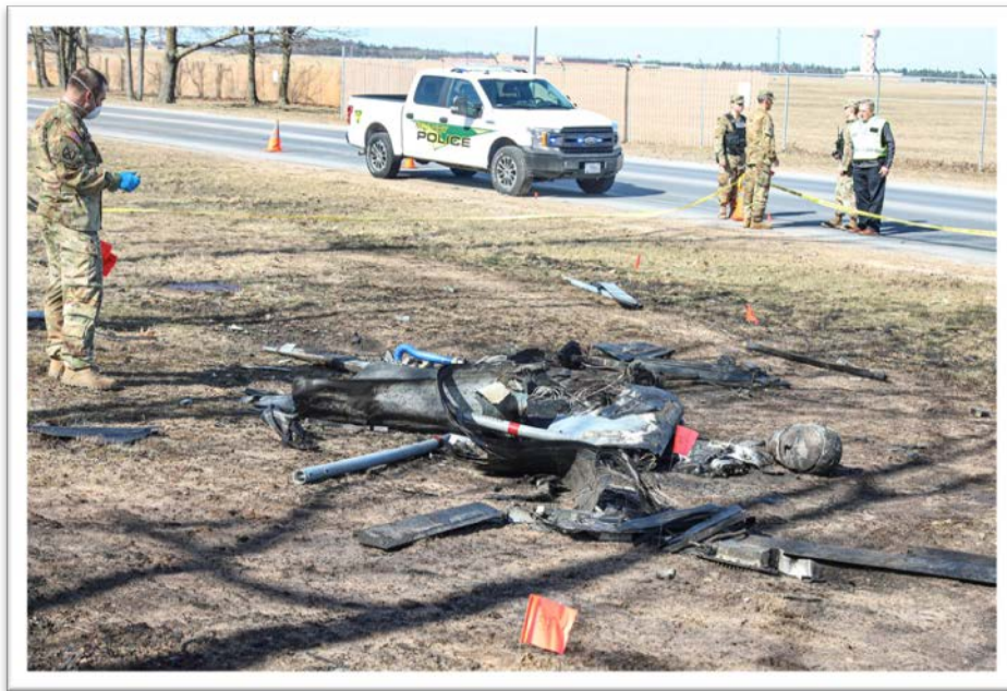
Figure 26 – The burnt wreckage of an RQ-7 Shadow drone at Fort Drum, New York
