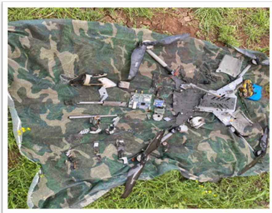
Figure 49 – Debris for an STM Kargu drone detonation
