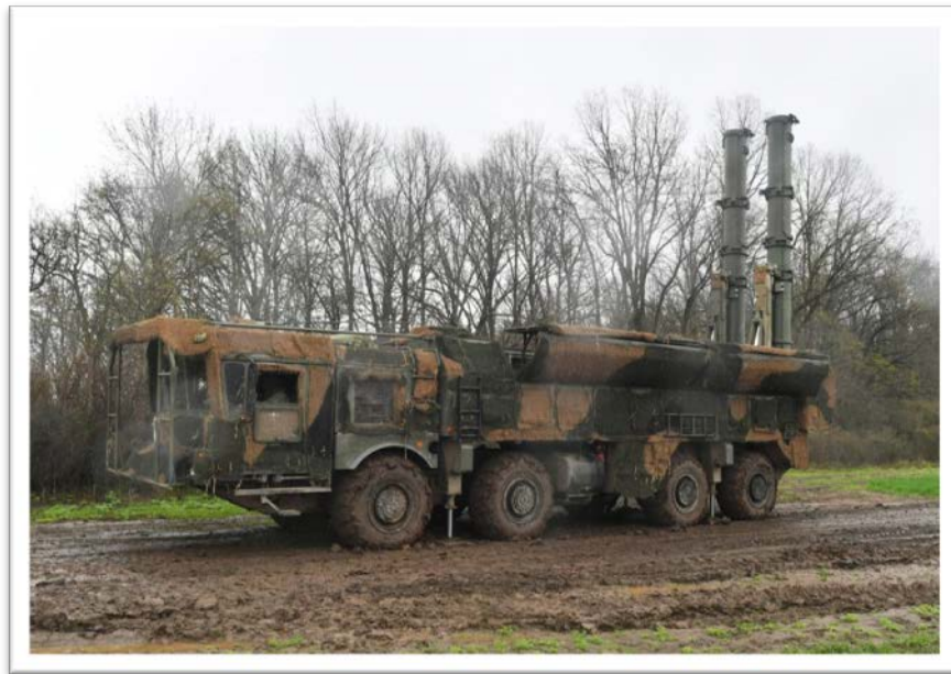
Figure 40 – A Russian Iskander missile launcher concealed with multi-spectral camouflage
