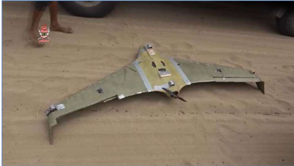
Figure 9 - Houthi Rased UAV recovered in September 2018 (photo: Lost Weapons)
