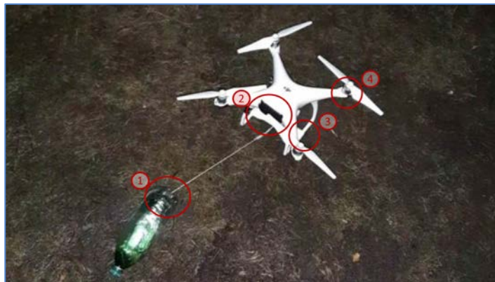
Figure 16 - Highlighted aspects of trigger mechanism (photo: USFIN)
