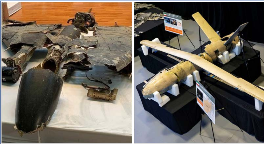
Figure 27 – Debris from low observable UAS used for Abqaiq attack and a Shahed 123 recovered by Saudi Arabia (photos: KSA)
