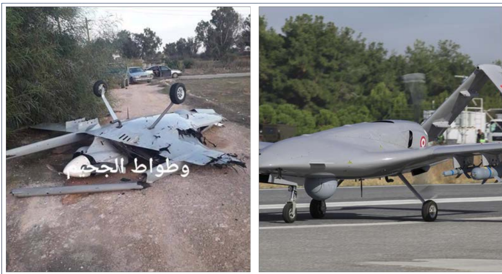
Figure 19 – Photo of the crashed TB2 (left) and an undamaged TB2 (right)
