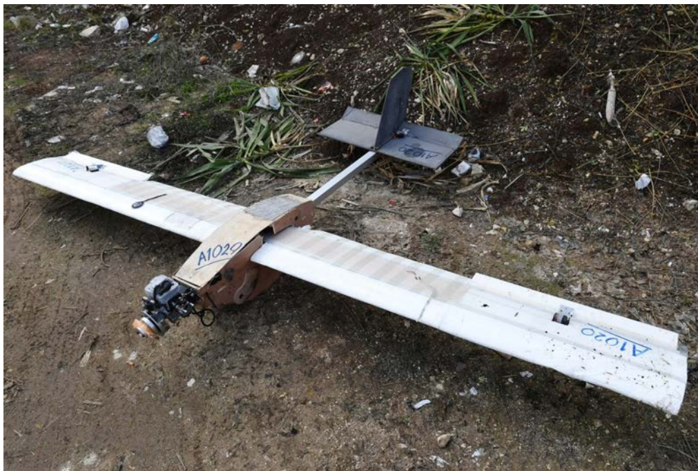
Figure 28 – Image of custom-made UAV shot down by Suqaylabiyah militia (photo: Mikhail Voskresensky)
